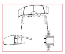
THE FRONT FAIRING IS NOT IN AN ACCEPTABLE POSITION IF ANY PART OF THE TUBES OF THE FRONT BUMPER ARE IN THE AREA 'A'.
