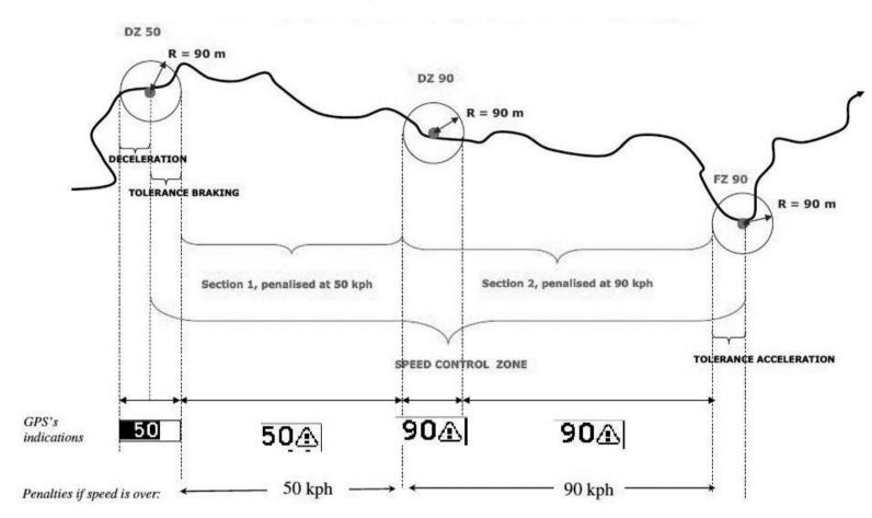
If the 2<sup>nd</sup> speed control zone has a lower speed limit than the 1<sup>st</sup> zone, the GPS shows it (white numbers on a black background) as soon as the competitor enters into the 90 m radius around the entry waypoint of the 2<sup>nd</sup> speed control zone. At the same time, the GPS still shows the ALARM SPEED triangle.
