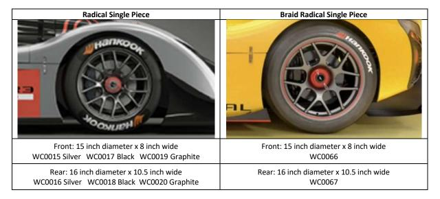
a) Only single piece wheels supplied by Radical Motorsport of the following specification are permitted.
