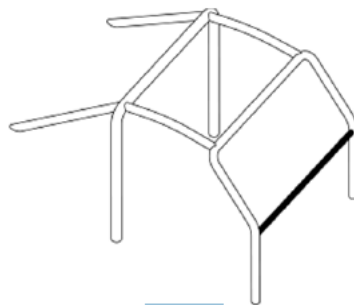
All black Tubes 40mm dia x 2.5mm
